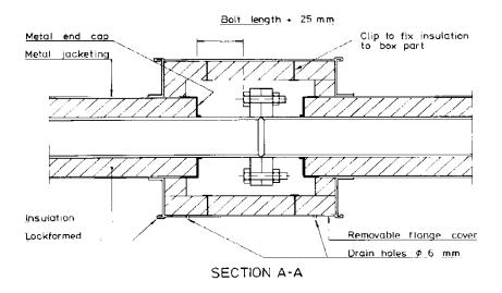
NOTE: Insulation to be fixed to box parts for easy removal and replacement
